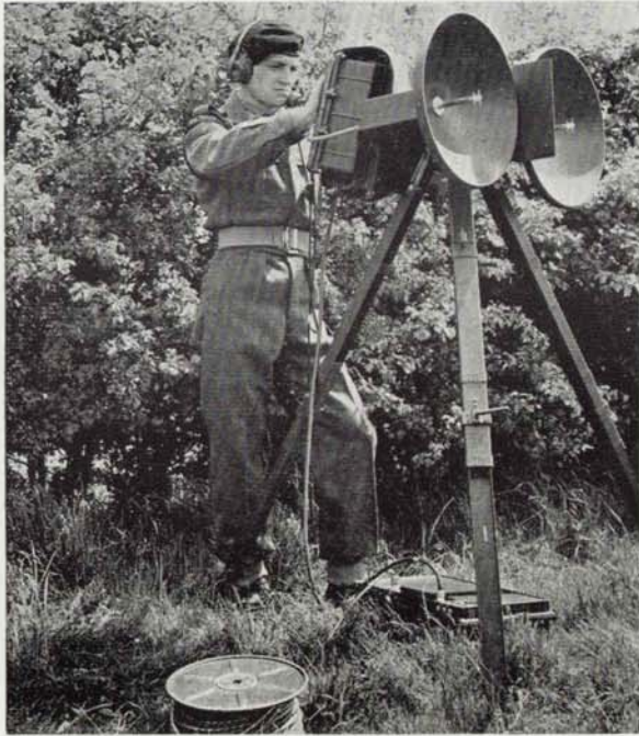
A Radio Relay Technician sets up a Radio Relay station.
