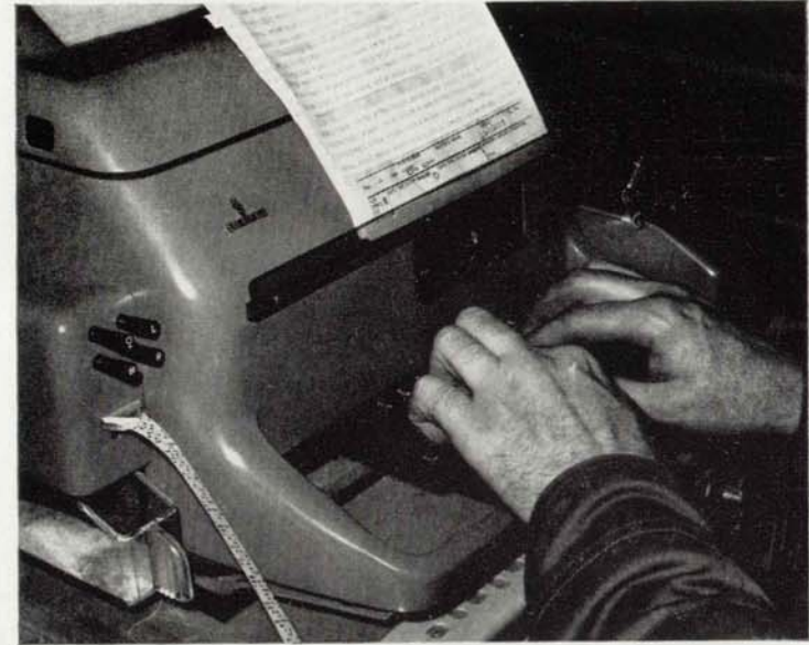
The skilled fingers of a Cipher Operator producing a perforated tape from a crypto copy on a T100 Teleprinter.
